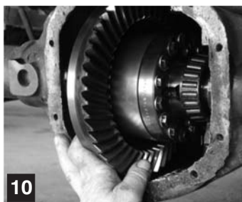
10 Install the NEKARTH and adjust the distance from CROWN to PINION;
