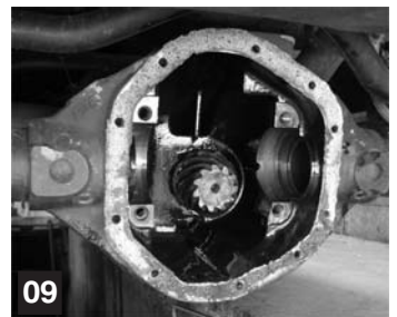
09 You don't need to remove the PINION from his place.
