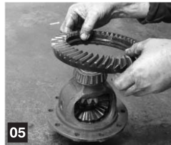
05 Pull out the original differential crown;
