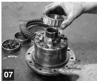
07 Preserving or replacing bearings/shims. Move then to NEKARTH;
