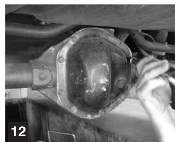
12 Replace the case cover; Replace the oil following the manufacturer recommendation for oil and quaitty.
