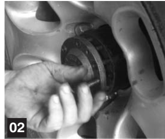
02 Pulling out and disconnect axles;
