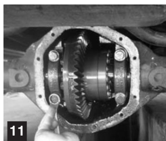
11 Place the NEKARTH at the case and fix the screws and bolts;
