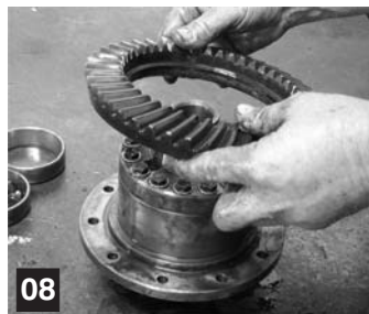
08 Move and Install the original crown at the NEKARTH;
